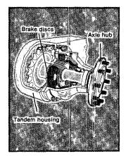
Four-wheel oil disc brakes are bathed in oil and sealed to the environment. They need none of the periodic adjustment and lining replacement typical of shoetype brakes. Each tandem set is activated by its own air circuit, so failure in one circuit still leaves half the original braking capacity. Choice of ROPS cabs or canopies, work lights, directional signals, other protective items are available for specific user needs.
