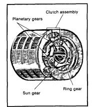
Direct drive power shift transmission was designed specifically for motor graders. It has no torque converter to cause lags or surges, just smooth no-clutch one-lever shifting with direct drive feel. Compact planetary gear sets provide high reduction in minimum space. large diameter clutch assemblies have high holding capacity. Plates are continuously lubricated and cooled by oil.
