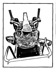
Work area visibility is excellent because of control location and frame design. An operator can work with increased confidence. While seated, he can see both ends of the blade and the ground ahead much better than on conventional machines. The Series G main frame is a single member all the way to the front axle. The top of the frame has none of the usual blade linkage obstructing the forward view.
